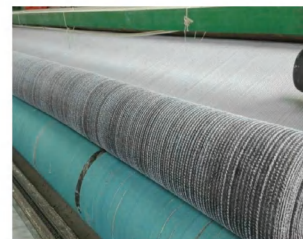
膨润土防水毯生产线 Geosynthetic Clay Liner production line
