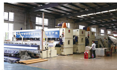
针刺土工布生产线 Needle punched geotextile production line
